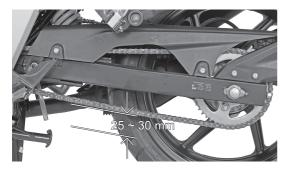
Check, clean, lubricate and adjust the drive chain in the following manner:
